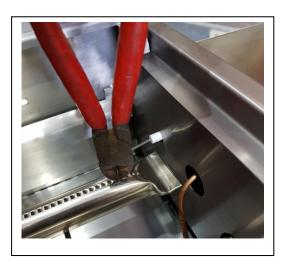
When there is no spark from the Piezo Ignitor, try cleaning the tip with a very fine sand paper. If it still does not spark try cutting the very tip off the Piezo with a sharp pair of pliers. If neither of these actions work then the Piezo might need replacing.
