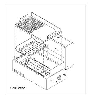
As the above diagram shows, the flame disperser clips in place on the left hand side of your Sovereign Flat/Grill BBQ, with the recessed/lowest part of the disperser (inclusive of larger drain holes) sitting over the fat tray (as shown above). Please ensure your disperser is installed in accordance with the above diagram.
